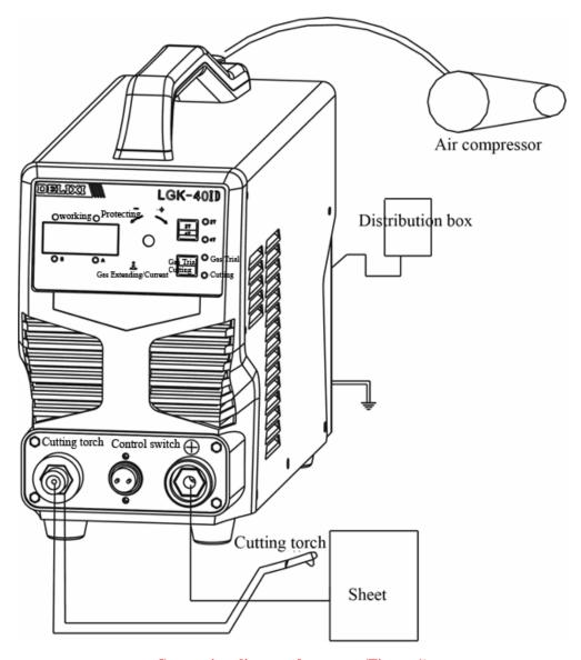
**Connection diagram for cutter (Figure 1)**
