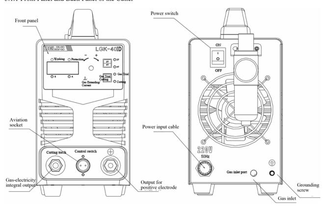
Figure 4 LGK-40ID Front Panel & Back Panel
